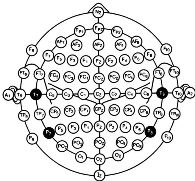
FIG. 1. Modified combinatorial nomenclature for the 10-10 system.
